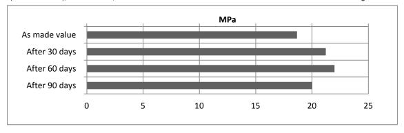
Lap shear strength versus heat ageing (ISO 4587) (typical average values)
